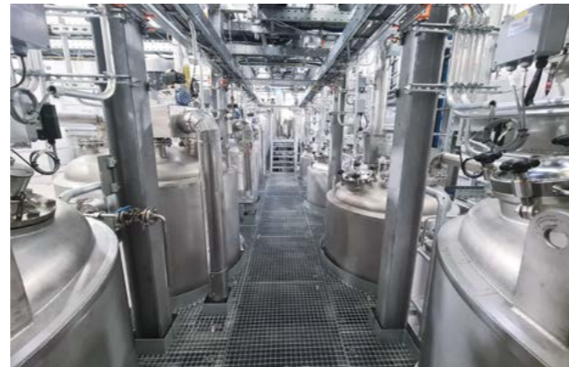
The finished extract can be stored in more than 20 tanks of differing sizes
